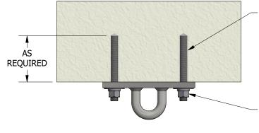
STAINLESS STEEL THREADED ROD WITH ADHESIVE OR EXPANSION ANCHOR (TYP 2 PLACES)
